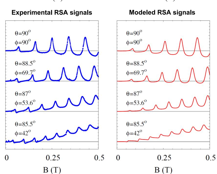
**Experimental verification of** model: experimental details as in the TRFR case and the repetition rate of the laser system is 80 MHz. All the parameters of the model, apart from the tilt angle, are the same for all modeled curves. Also, to account for the inhomogeneous ensemble broadening of the hole gfactors, the modeled result was averaged according to Gaussian distribution of g-factors.
