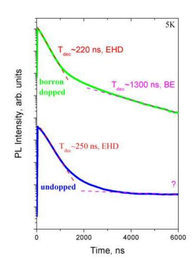
← PL decays recorded for the doped and undoped QWs with x=4.5% at 5K. Spectral region corresponds to BE<sub>TO</sub> and EHD<sub>TO</sub> emission lines. For both samples EHD lifetime can be determined. For the doped one BE decay time well resolved as well.
