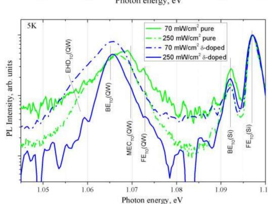
Appearance of BE emission and suppression of EHD emission for the boron doped QW with x=4.5%. Spectra recorded at steady-state excitation (excitation densities shown at the figures). Temperature is equal to 10K for upper figure and 5K for bottom one.
